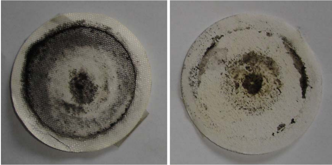
Figure 16 Comparison of particulate samples (undiluted exhaust gas upstream filter passing through a Pallflex 47mm filter during the total cycle. Left: Diesel fuel. Right: B70 biodiesel blend.
