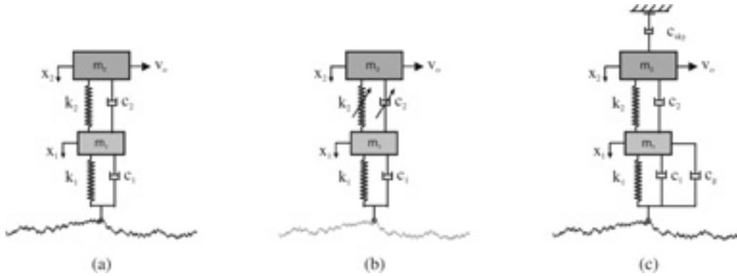
Figure 1. Vehicle models: (a) linear model, (b) piecewise linear model, and (c) sky-hook model.
