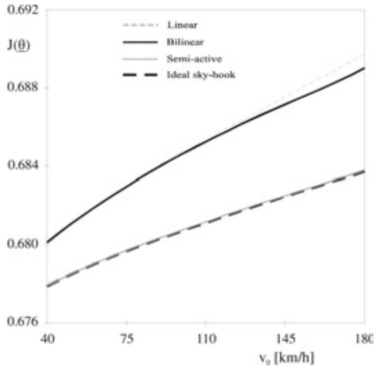
Figure 15. Comparison of performance index values for quarter-car models with a linear damper, a bilinear damper, a nonlinear sky-hook, and an ideal sky-hook damper.
