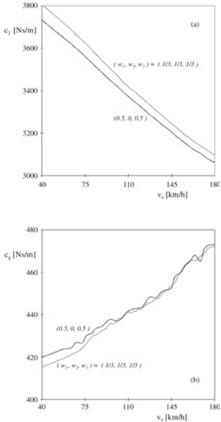
Figure 13. Optimum values for (a) the suspension damping coefficient  $c_2$  and (b) the damping coefficient  $c_g$ , for an ideal sky-hook car model.
