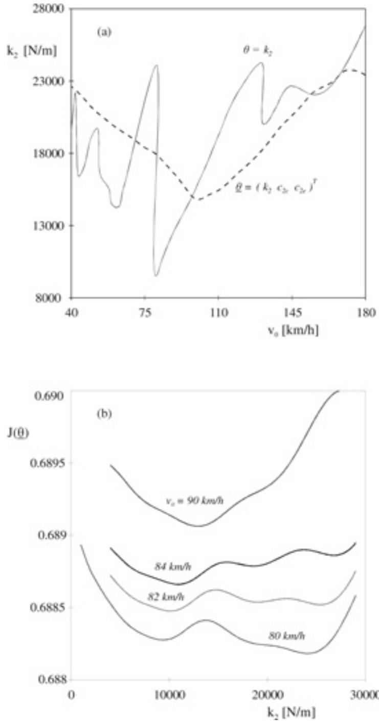
Figure 12. (a) Optimum values for the suspension stiffness coefficient  $k_2$  and (b) performance index, for a quarter-car model with bilinear suspension damper.
