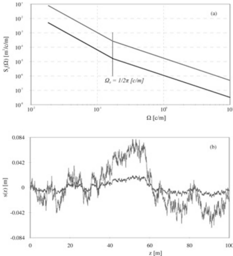
Figure 3. (a) Response spectra of typical roads and (b) profiles of a good-quality road and a poor-quality road.
