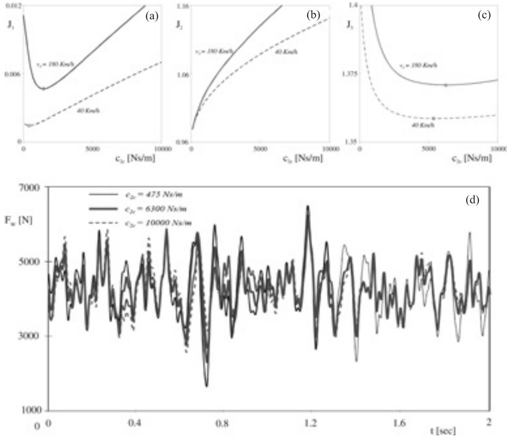
Figure 11. (a)–(c) Dependence of the functions  $J_n$  ( $n = 1, 2, 3$ ) on the suspension damping coefficient  $c_{2e}$ , for the two extreme values of the car speed  $v_0$ . (d) History of tire force  $F_w$ , obtained at  $v_0 = 180 \text{ km h}^{-1}$  for three selected values of the suspension damping coefficient  $c_{2e}$ .
