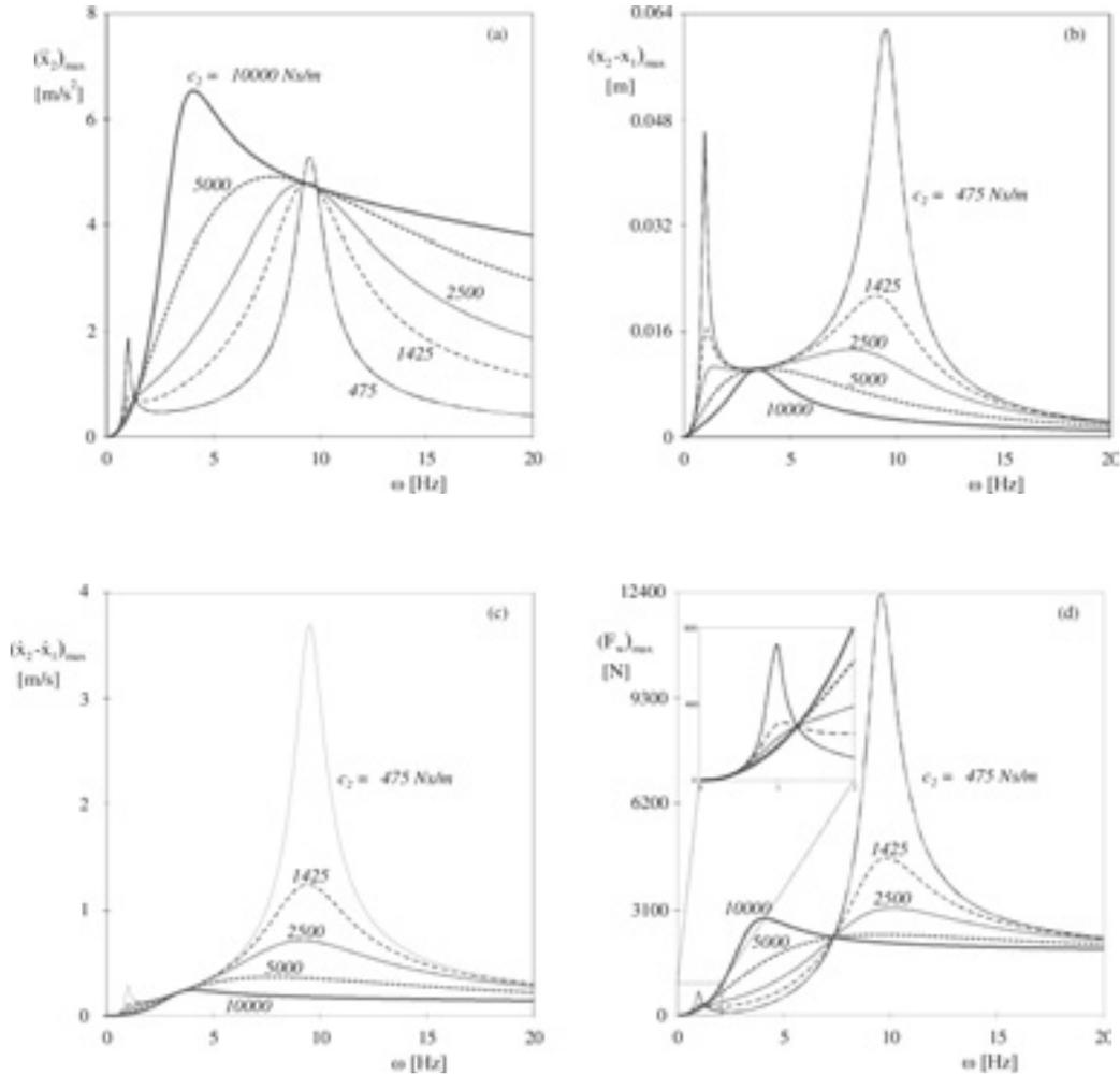
Figure 6. Response spectra of linear car models for (a) the vehicle body acceleration  $\ddot{x}_2$ , (b) the relative displacement  $x_2 - x_1$ , (c) the relative velocity  $\dot{x}_2 - \dot{x}_1$ , and (d) the tire force  $F_w$ .
