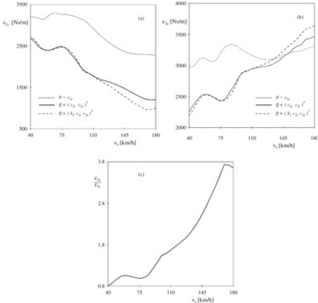
Figure 9. Optimum values for the suspension damping coefficient in (a) compression and (b) extension, for a quarter-car model with bilinear suspension damper. (c) Dependence of the suspension damping coefficient ratio  $c_{2e}/c_{2c}$  on the horizontal vehicle speed  $v_0$ .
