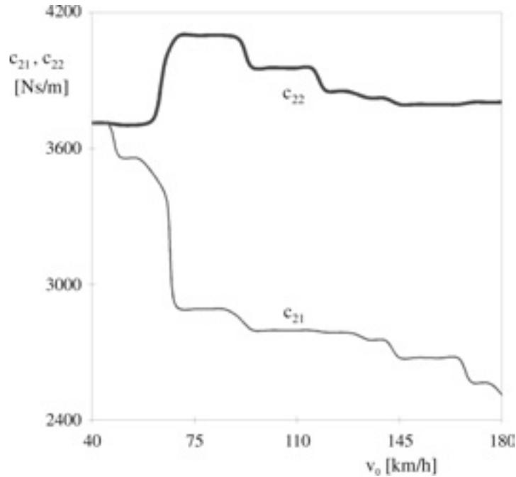
Figure 14. Optimum values for the suspension damping coefficients  $c_{21}$  and  $c_{22}$  of a nonlinear sky-hook car model.
