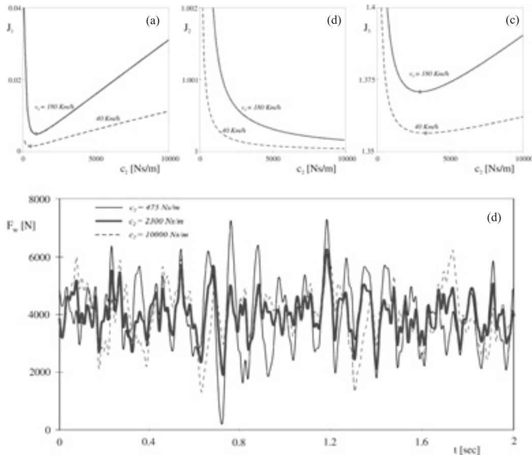
Figure 7. (a)–(c) Dependence of the functions  $J_n$  ( $n = 1, 2, 3$ ) on the suspension damping coefficient  $c_2$ , for the two extreme values of the vehicle speed  $v_0$ . (d) History of tire force  $F_w$ , obtained at  $v_0 = 180 \text{ km h}^{-1}$  for three selected values of the suspension damping coefficient  $c_2$ .
