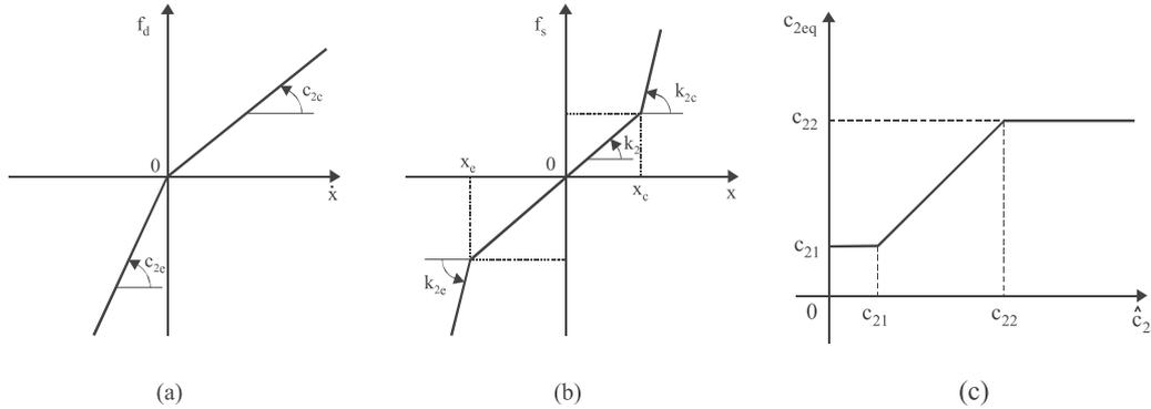
Figure 2. (a) Force characteristics of suspension damper. (b) Restoring force of suspension spring. (c) Equivalent suspension damping coefficient of sky-hook model.
