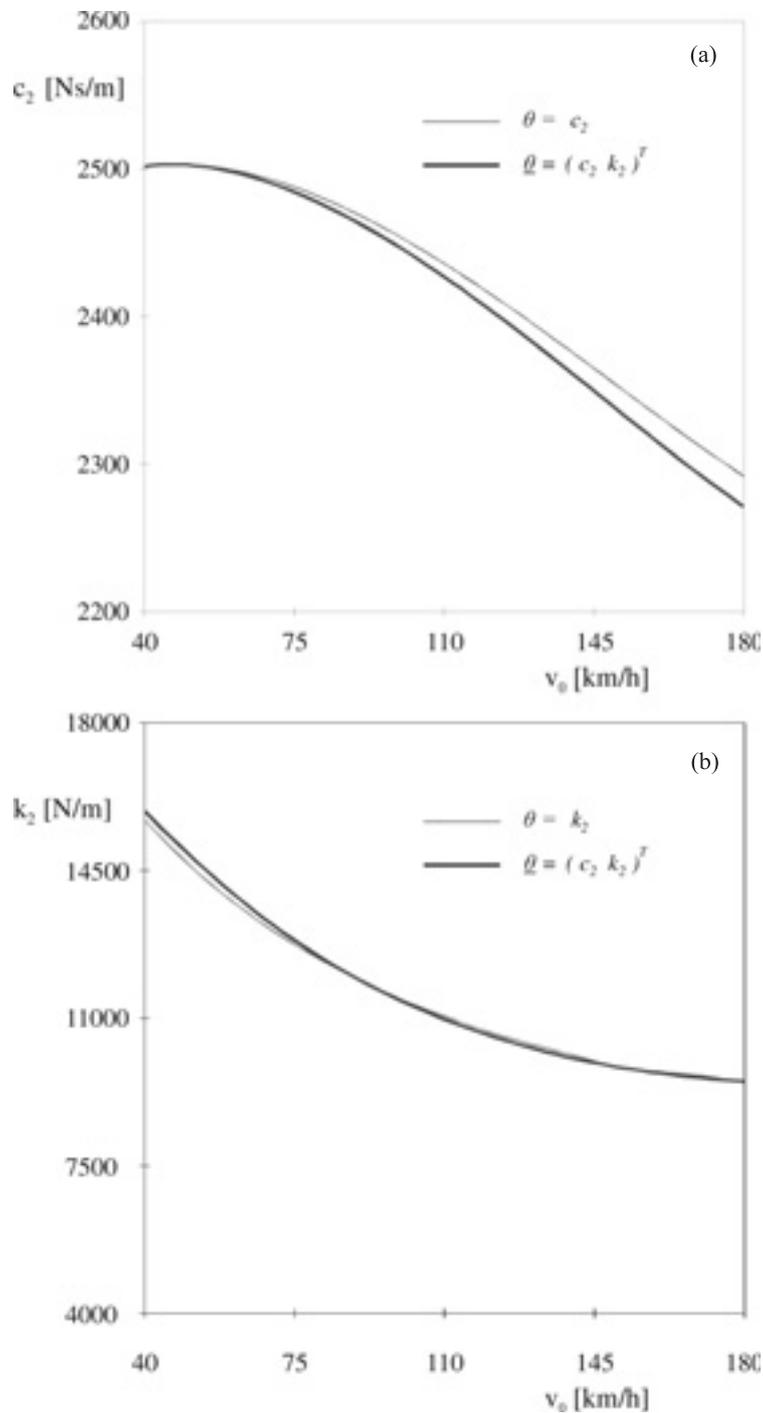
Figure 4. Optimum values for (a) the suspension damping coefficient  $c_2$  and (b) the suspension stiffness coefficient  $k_2$ , for a quarter-car model with linear suspension damper.
