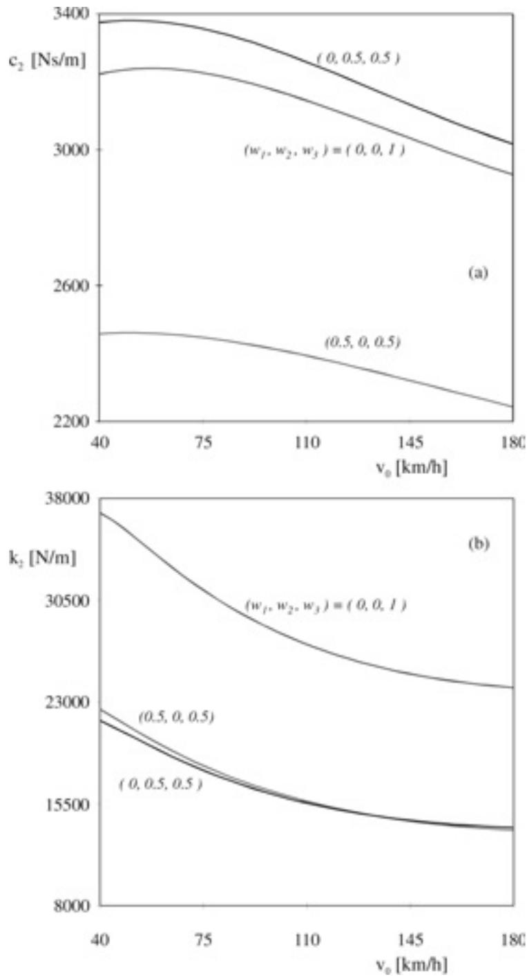
Figure 5. Optimum values for (a) the suspension damping coefficient  $c_2$  and (b) the suspension stiffness coefficient  $k_2$ , for different values of the weighting coefficients.
