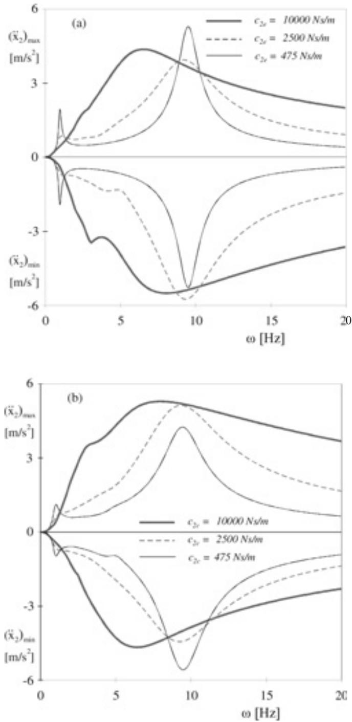
Figure 10. Response spectra (maximum and minimum values) of the vehicle body acceleration  $\ddot{x}_2$  for quarter-car models with dual-rate dampers: (a)  $c_{2e} = 475$  Ns m<sup>-1</sup> and several values of  $c_{2c}$ ; (b)  $c_{2e} = 1425$  Ns m<sup>-1</sup> and several values of  $c_{2c}$ .
