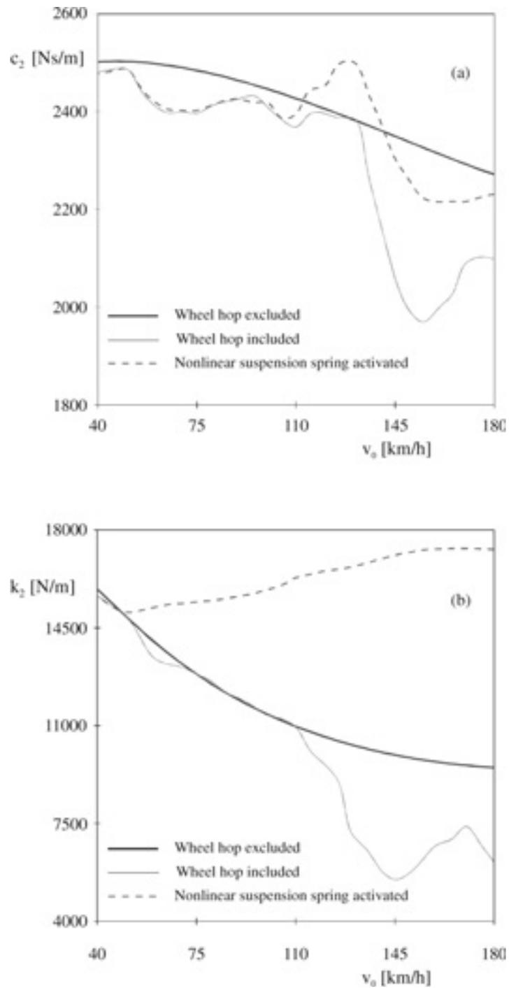
Figure 8. Optimum values for (a) the suspension damping coefficient  $c_2$  and (b) the suspension stiffness coefficient  $k_2$ , of a quarter-car model with wheel hop and nonlinear spring.
