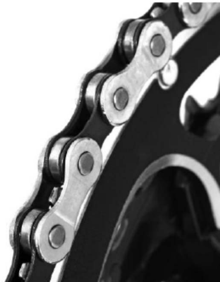
A rolling chain on a sprocket. Source: Shutterstock.
