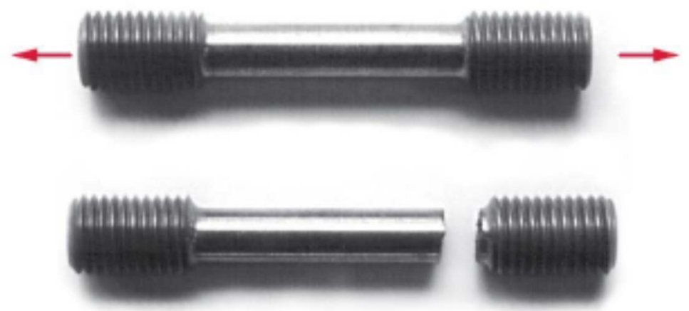
A Tensile Test Specimen of Brittle Cast Iron Before and After Fracture
